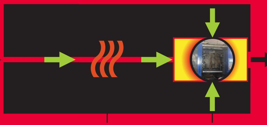
The plastic beads are heated to a temperature of 580 F/304 C to melt the plastic into a liquid.
